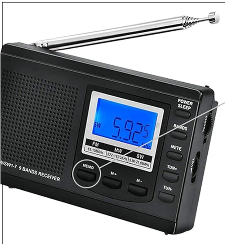
Figure 6.2: The radio's display shows the current frequency and band. The MEMO button and M+/M- buttons are used for managing station presets.
