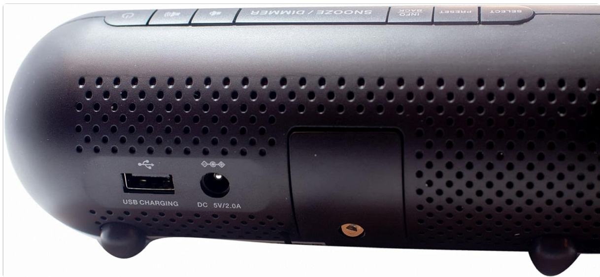
Figure 3: Rear view of the unit, highlighting the USB charging port and the DC 5V/2.0A power input connection.
