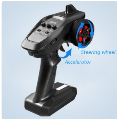
Image: A close-up of the remote control, indicating the steering wheel and accelerator trigger for controlling the RC car.
