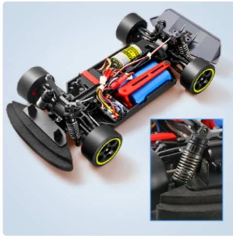
Image: A detailed view of the RC car's shock absorber, indicating its role in suspension and handling.
