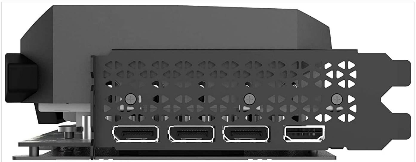
Image: Display output ports on the graphics card, including DisplayPort and HDMI.
