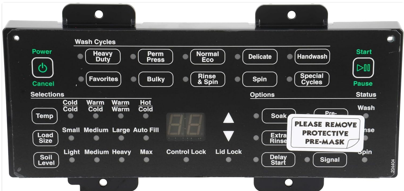
Image: Front view of the ALLIANCE LAUNDRY SYSTEMS Control Board and Overlay Assembly (204074P), showing the user interface with buttons for Power, Start/Pause, Wash Cycles (Heavy Duty, Perm Press, Normal Eco, Delicate, Handwash, Favorites, Bulky, Rinse & Spin, Spin, Special Cycles), Selections (Temp, Load Size, Soil Level), Options (Soak, Extra Rinse, Delay Start, Signal), and Status indicators. A protective film with "PLEASE REMOVE PROTECTIVE PRE-MASK" is visible on the right side.
