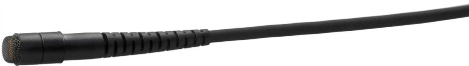
Figure 1: Close-up view of the DPA 4660 CORE Heavy-duty Omnidirectional Lavalier Microphone, showing the microphone capsule and the robust cable.
