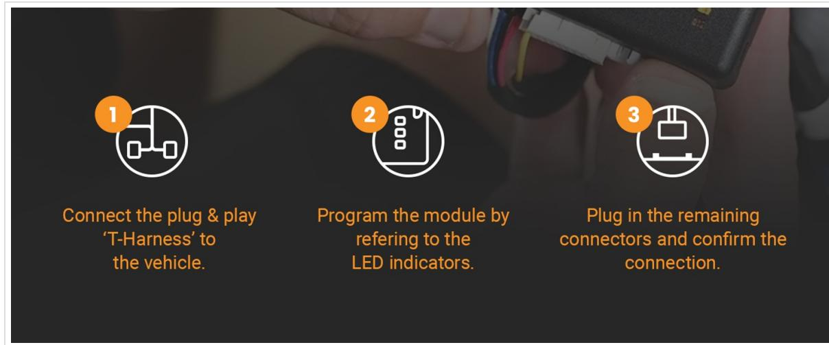
A visual guide illustrating the three primary steps for installation: connecting the T-Harness to the vehicle, programming the module using LED indicators, and securing all remaining connections.
