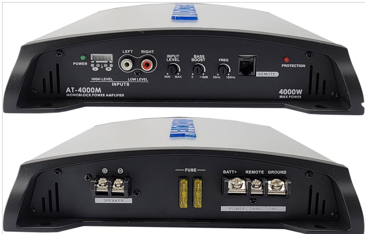
Image: Overview of the amplifier's input/control panel and power/speaker connection panel.
