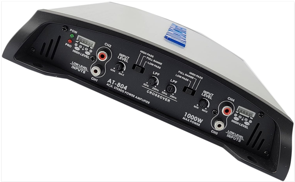
Image: Front view of the Audiotek AT804 amplifier, displaying the input level controls, crossover settings (High Pass, Full Range, Low Pass), and RCA/High-Level inputs for channels 1-4.
