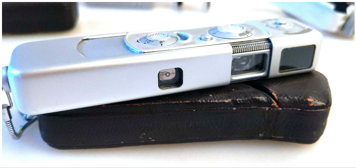
Figure 2.2: Detailed view of the MINOX B camera's front, highlighting the lens, viewfinder, and the exposure and focus dials on the top surface. The camera rests on its leather case.
