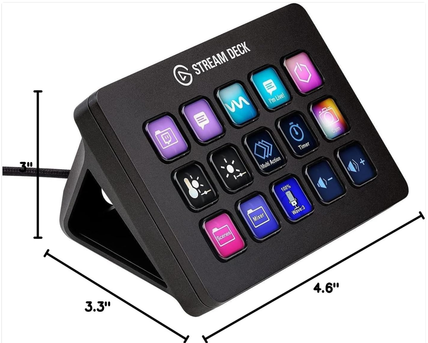
Figure 11: Physical dimensions of the Elgato Stream Deck MK.2.
