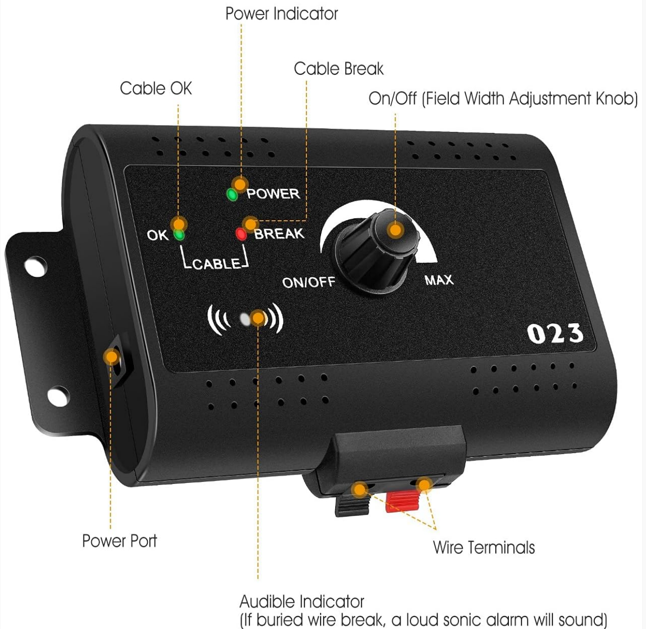
Image: A detailed view of the transmitter unit, highlighting its features: Power Indicator, Cable OK/Break Indicator, On/Off (Field Width Adjustment Knob), Power Port, Wire Terminals, and Audible Indicator.
