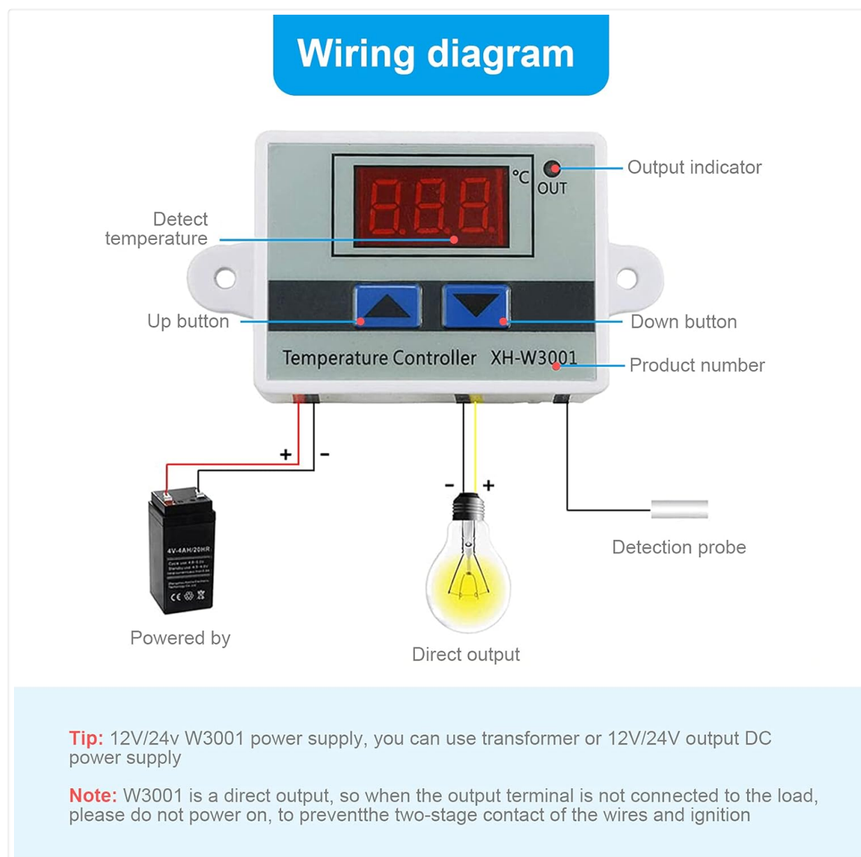
Figure 4: Setting temperatures on the XH-W3001. This image illustrates the display and buttons used for adjusting the start and stop temperature settings.
