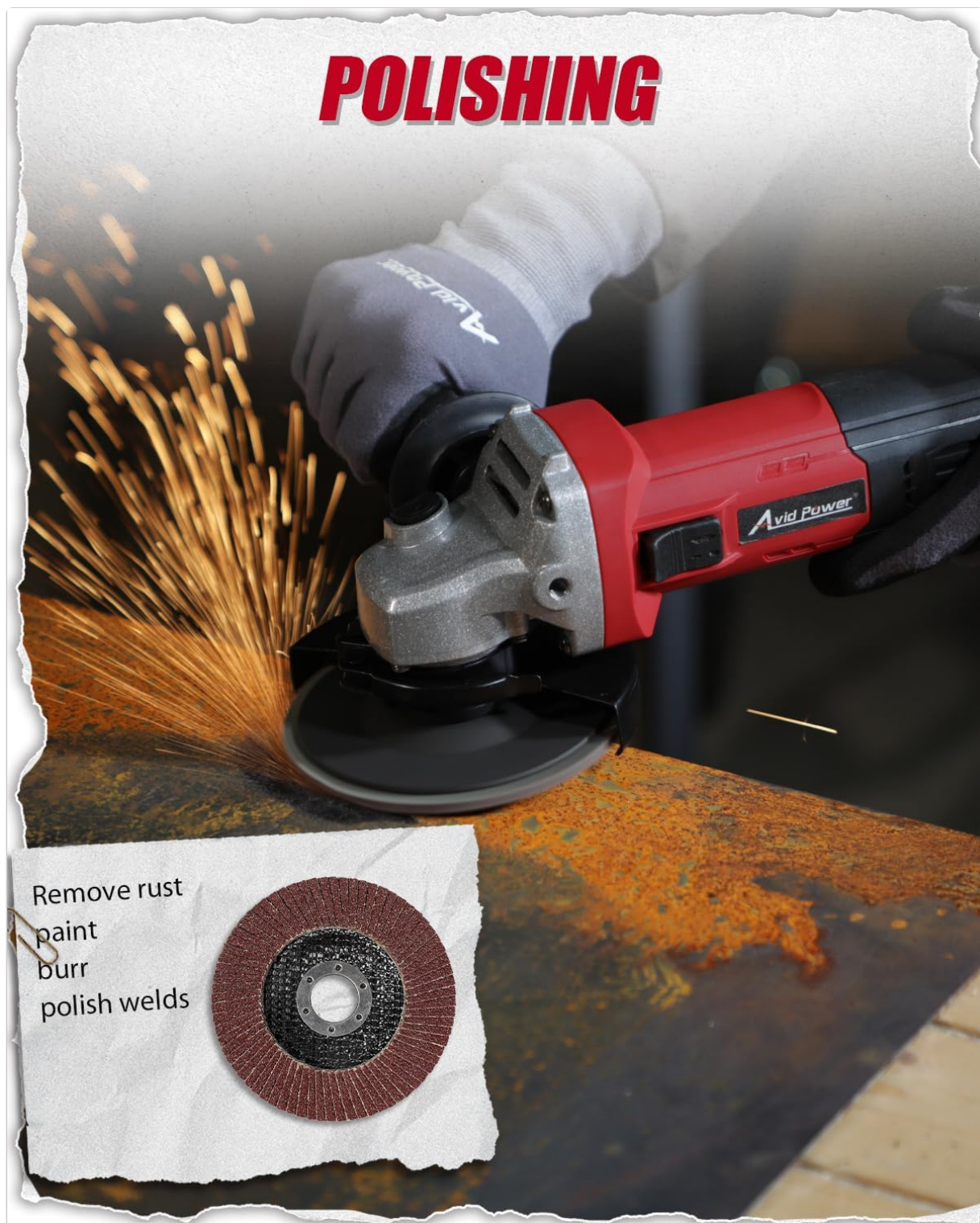
Figure 5.5: The angle grinder utilizing a flap disc to polish a rusty metal surface, demonstrating its effectiveness in surface preparation and rust removal.
