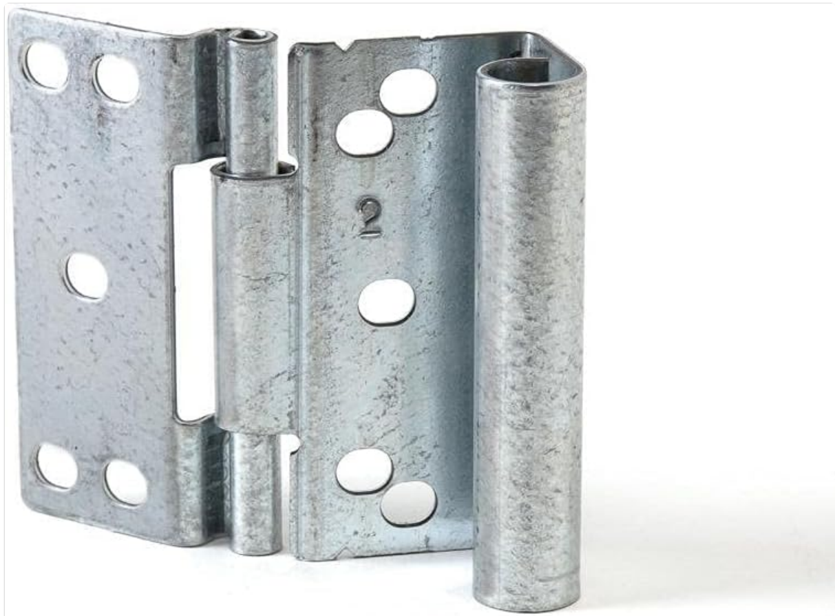
Figure 1: Front view of the Wayne Dalton Anti-Pinch Hinge #2. This galvanized steel hinge is designed for durability and features a unique shape to accommodate the garage door roller and prevent finger pinching between door sections.
