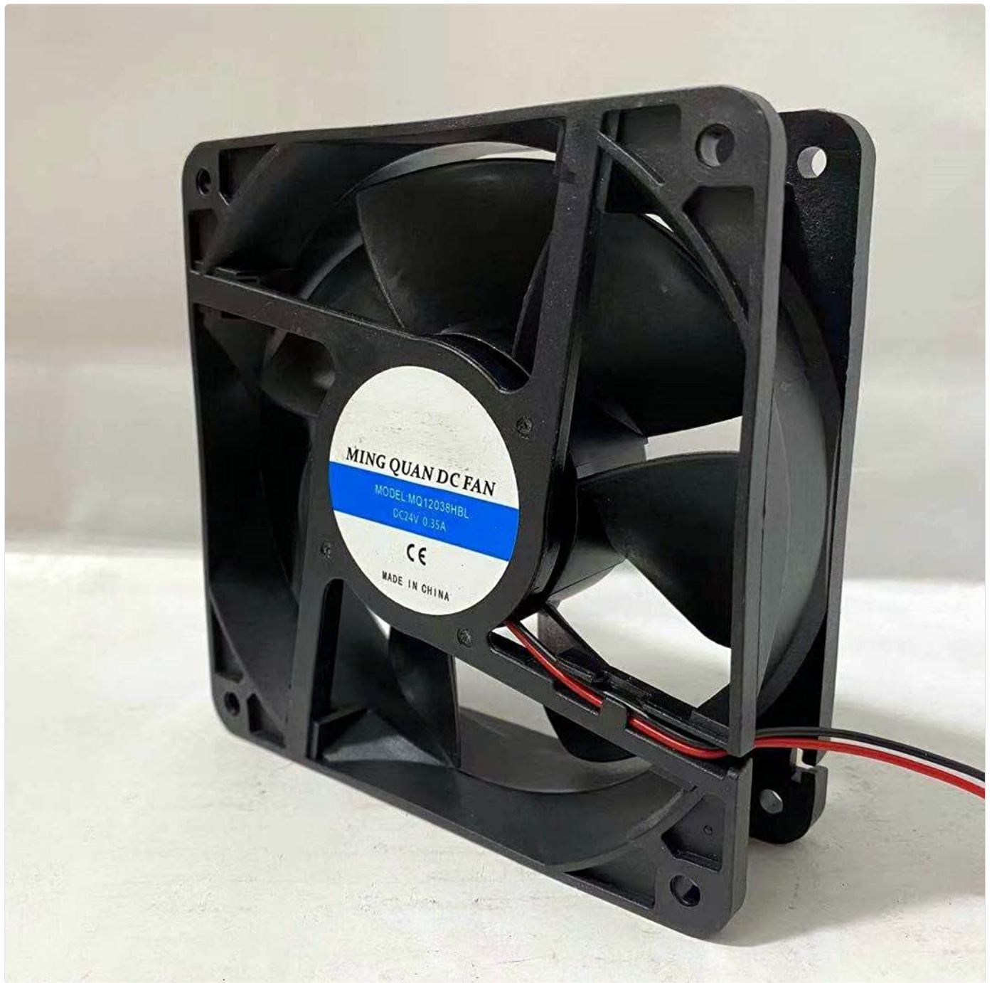
Figure 2.1: Front view of the ELOMILE MQ12038HBL DC fan, highlighting the central label with model information.
