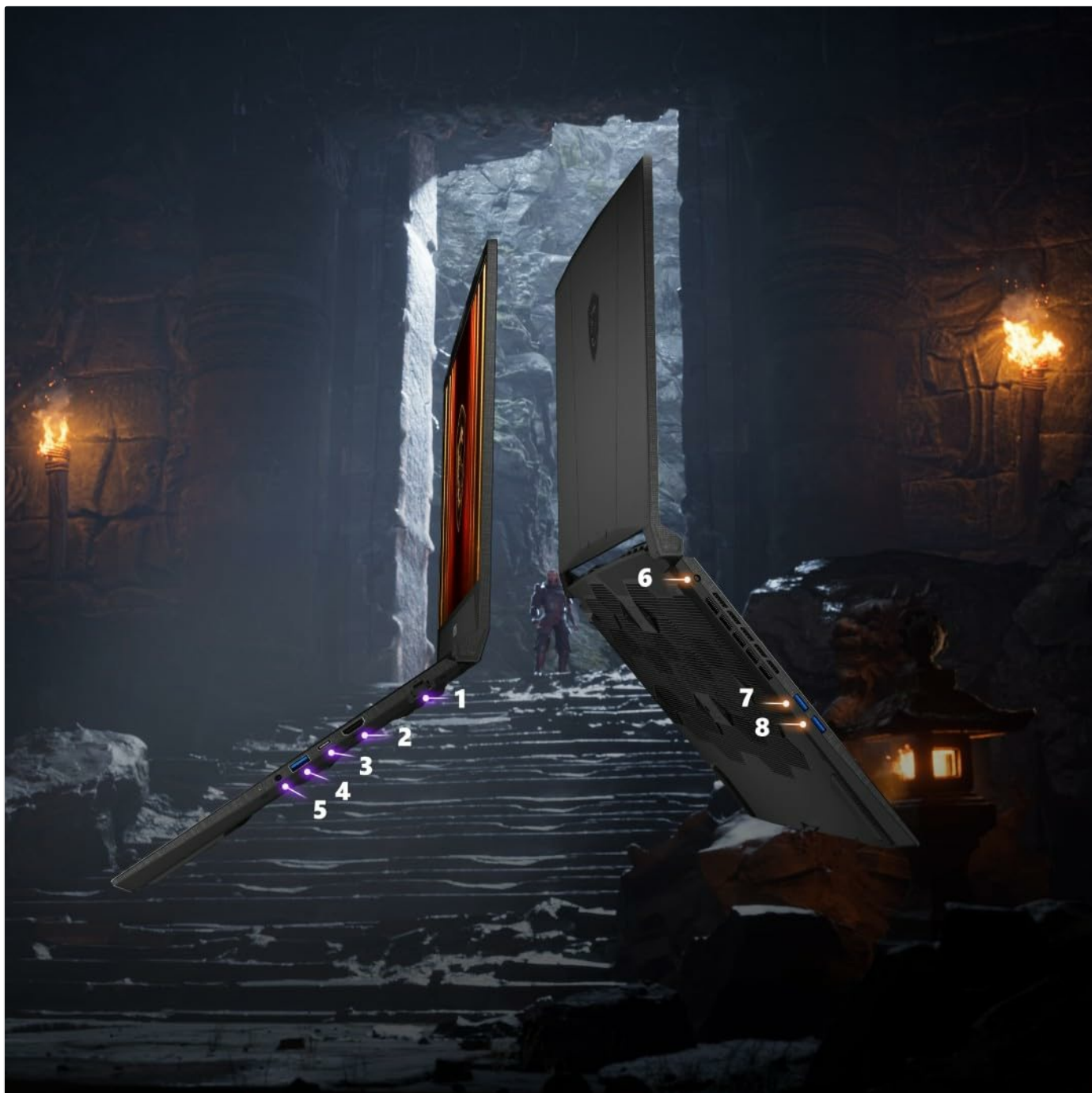
Figure 2.2.1: Side view of the MSI Katana 15 HX laptop, illustrating the location of various input/output ports and indicators. These include USB Type-C, HDMI 2.1, USB Type-A, audio jacks, and the power input.
