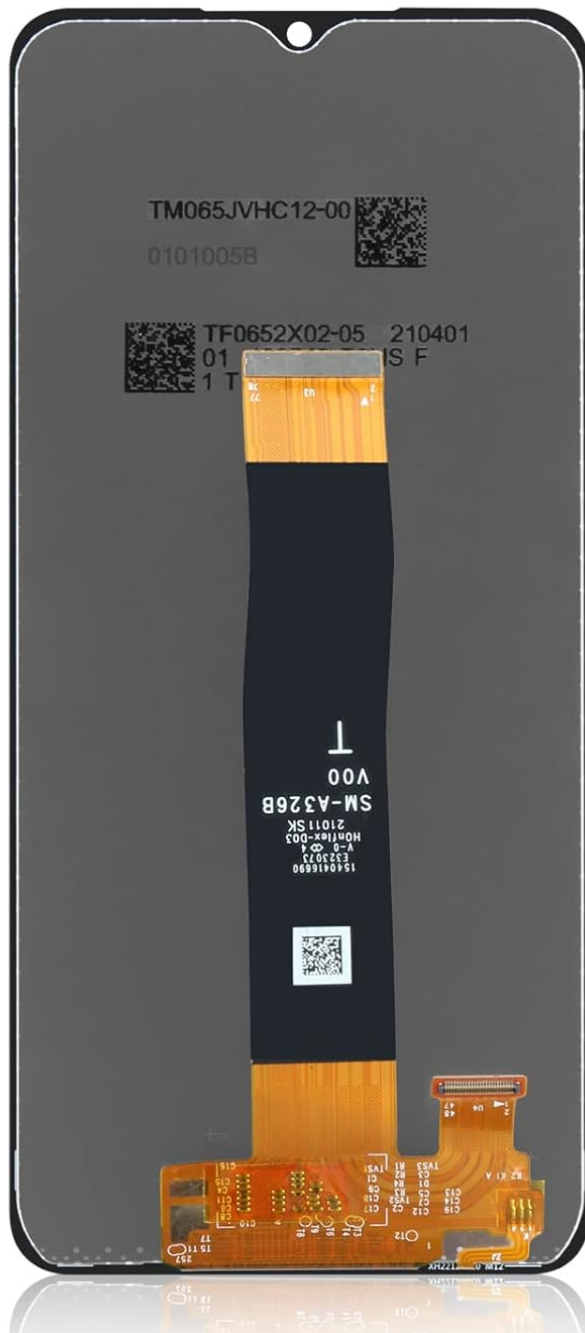
Image: Close-up of Samsung Galaxy A32 5G screen flex cable and connector details.
