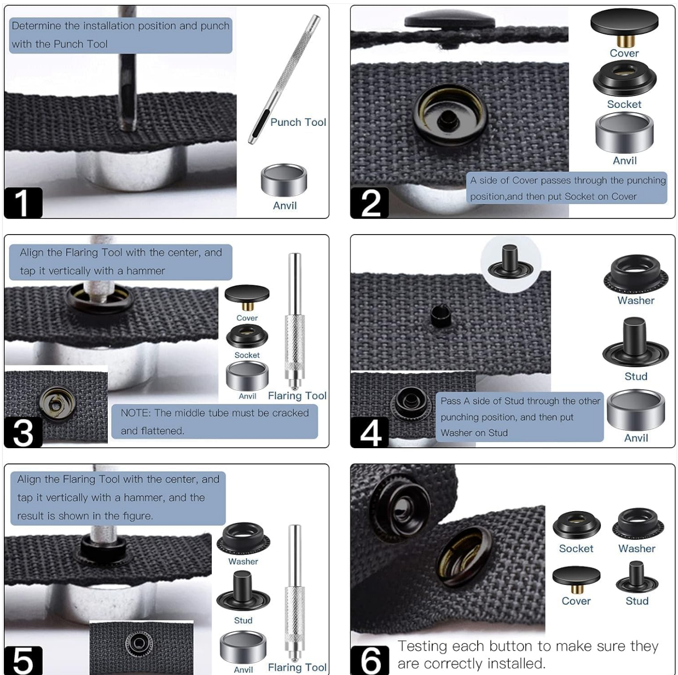
Image 4.1: Visual step-by-step guide for snap fastener installation.
