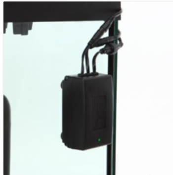
Image 4.2: The control box, typically mounted outside the aquarium, featuring an LED indicator.
