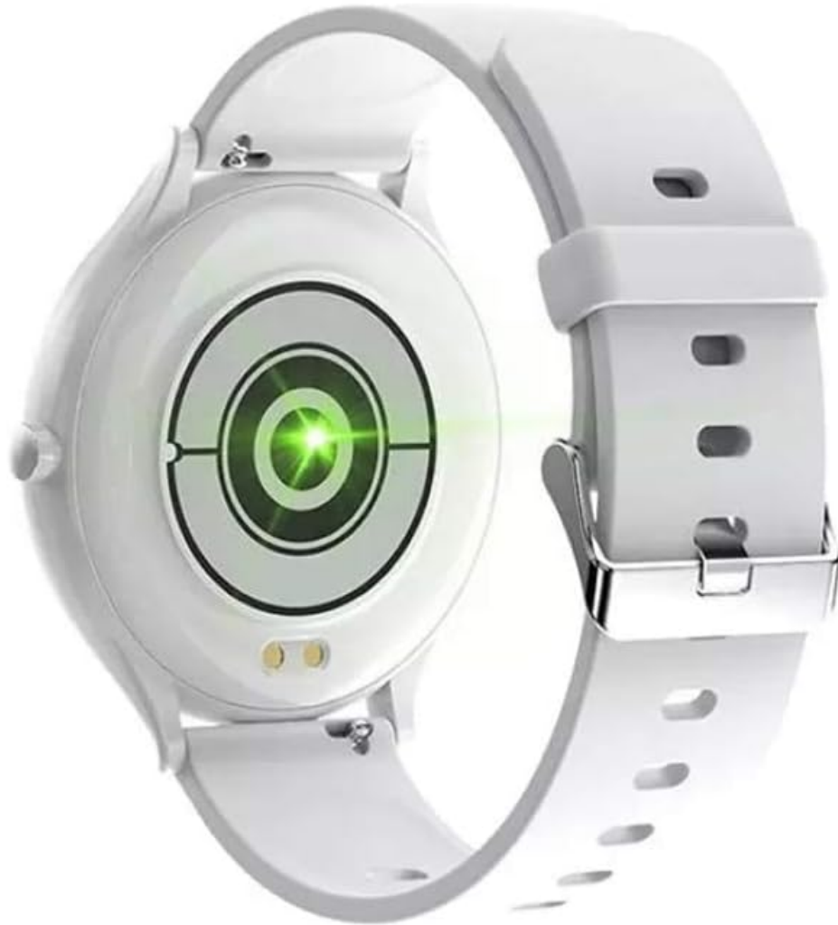
Figure 4: The optical heart rate sensor on the back of the watch ensures accurate readings.
