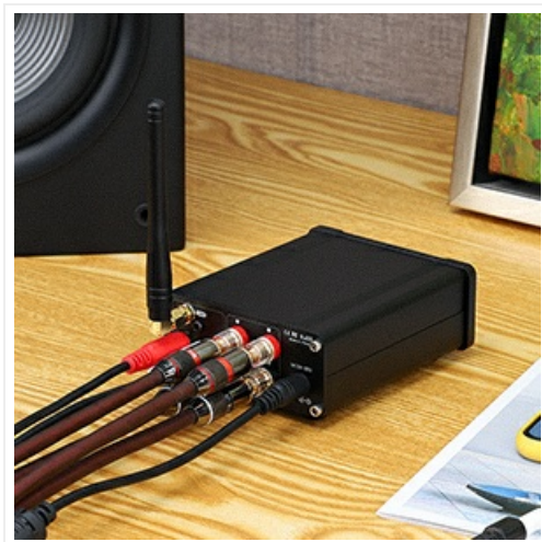
Image 5.1: Rear panel of the amplifier with Bluetooth antenna, RCA cables, speaker wires, and power adapter connected.
