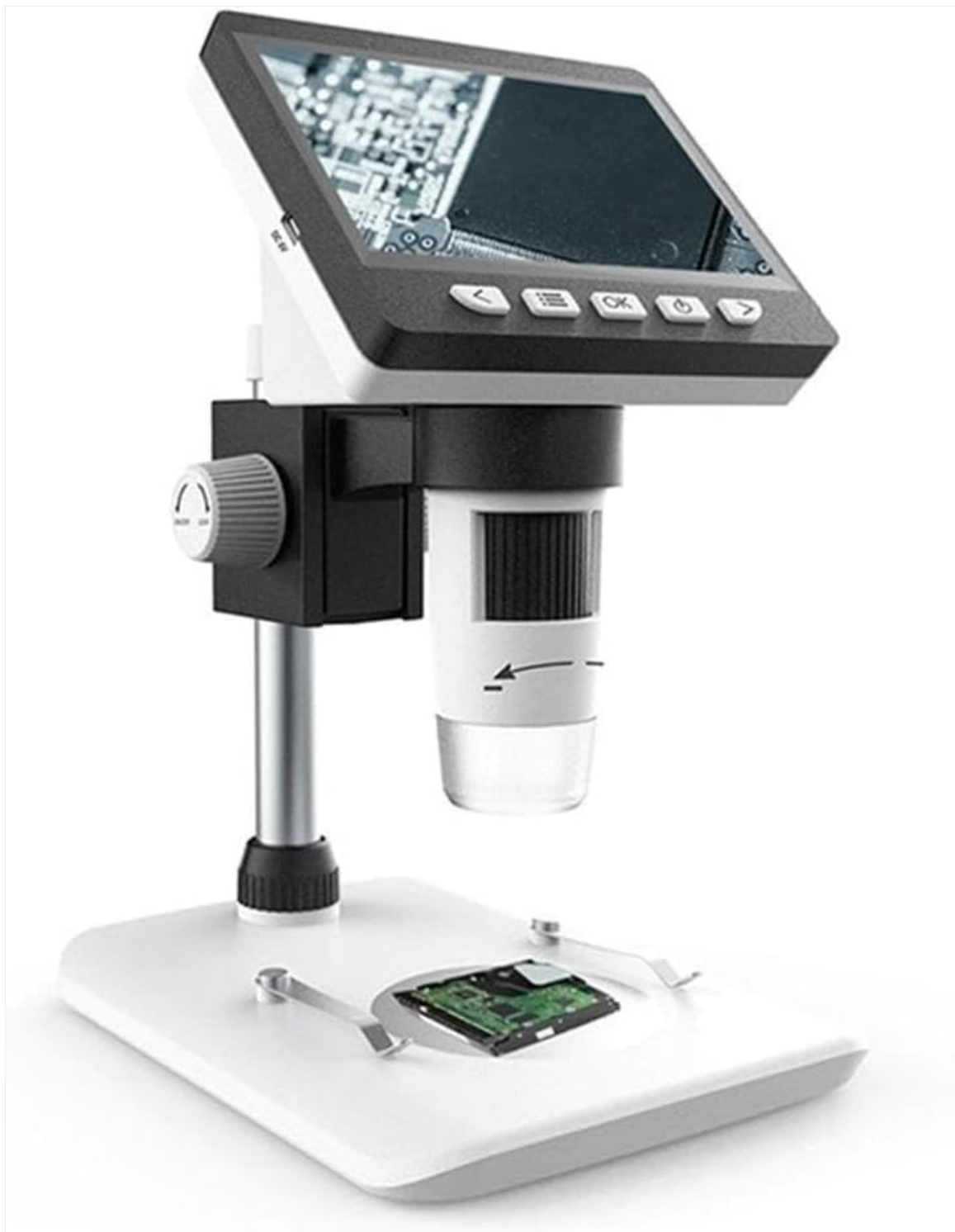
Figure 2: The Inskam 307 Digital Microscope in use, examining a circuit board on its object stage.
