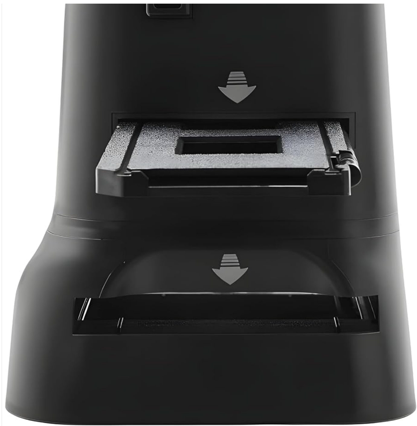
Figure 4.4: Side view of the Reflecta x66-Scan, highlighting the dedicated slot for 120 medium format film. This slot allows for direct insertion of the 120 film holder.
