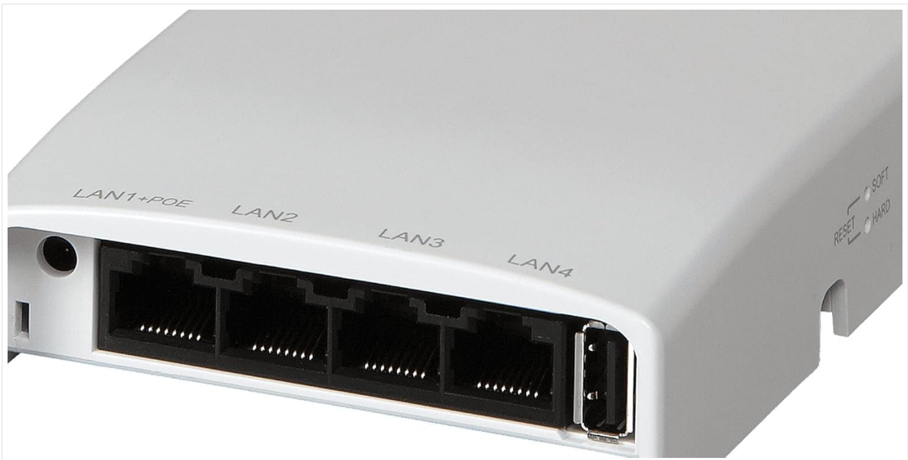
Figure 3: Close-up view of the front panel, showing LAN1+PoE, LAN2, LAN3, LAN4 ports, and a USB port.
