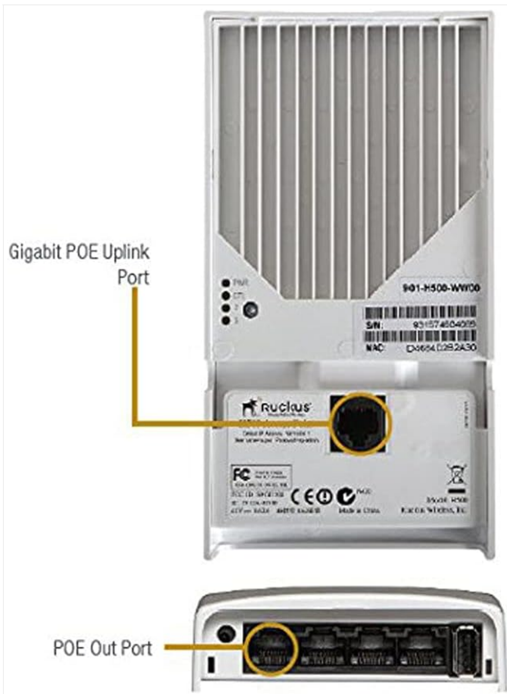
Figure 4: Rear view of the Ruckus ZoneFlex H500, highlighting the Gigabit PoE Uplink Port and reset buttons.
