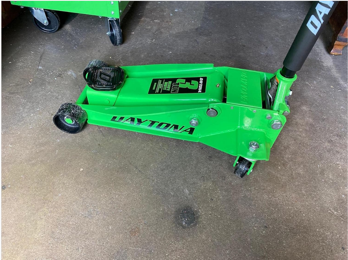
Figure 1: Overview of the Daytona 3 Ton Professional Rapid Pump Floor Jack. This image shows the jack in its lowered position, highlighting its compact design and green finish.
