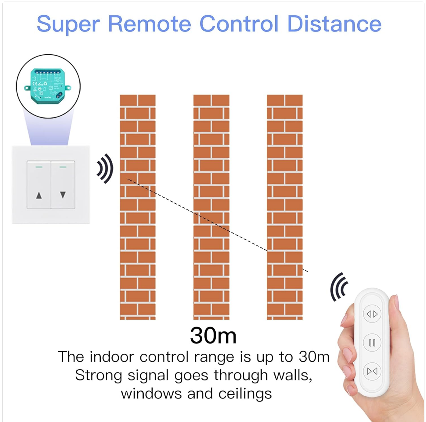
Figure 6: Illustration demonstrating the effective remote control range of up to 30 meters indoors, capable of transmitting signals through common building materials.
