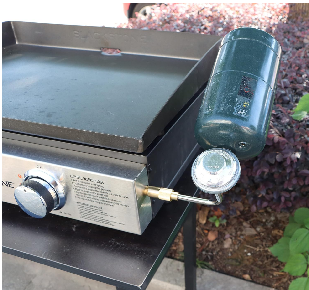
Image 5.3: Close-up view of the regulator connected to the griddle and propane tank.
