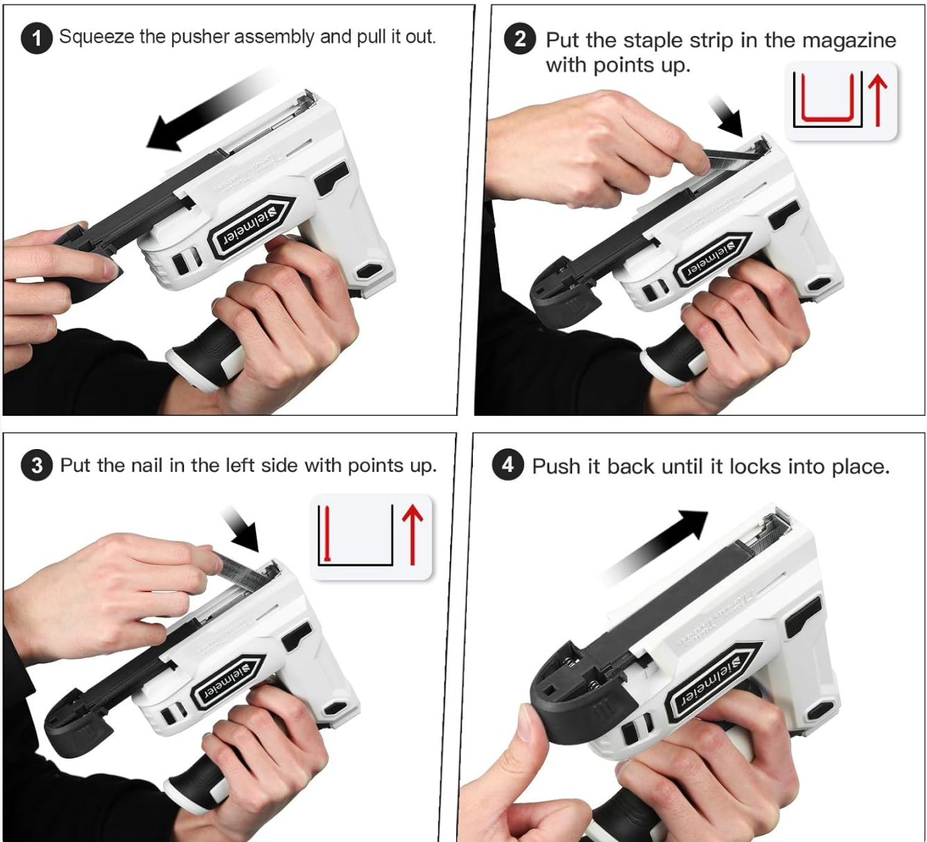
Figure 3: Steps for loading staples and nails.
