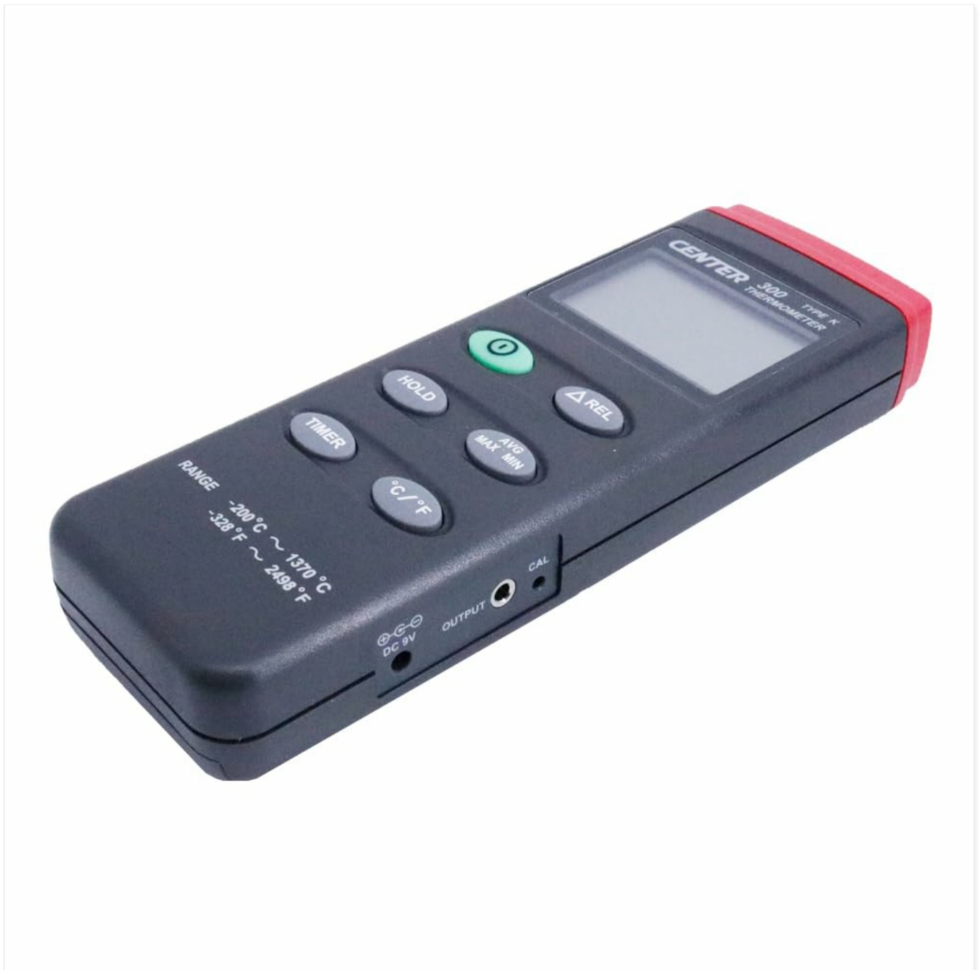
Figure 5: Side view of the thermometer, showing the DC 9V input and data output ports.
