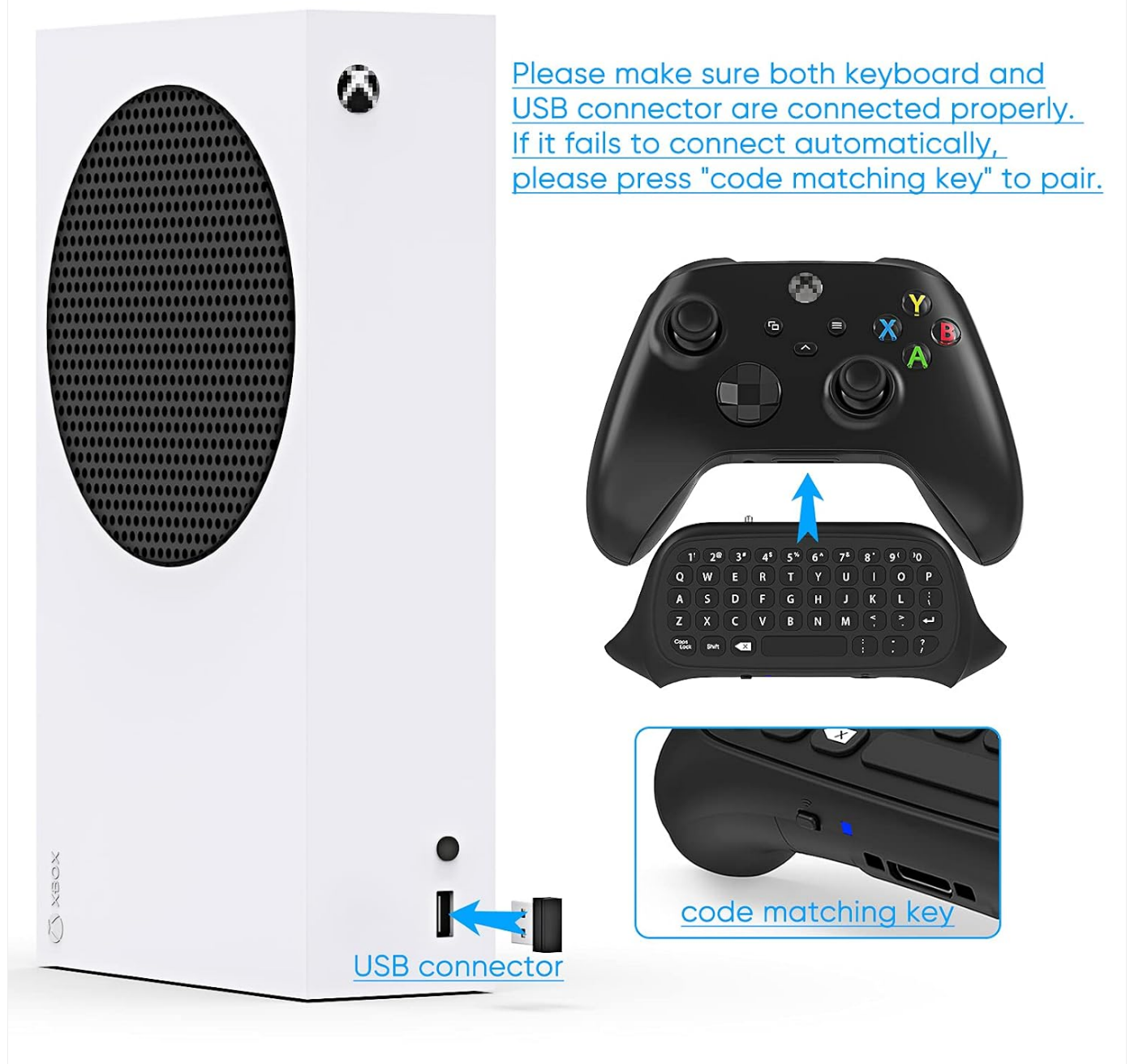
Figure 4: Inserting the 2.4G USB receiver into the console.
