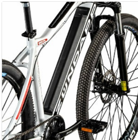
Figure 4.1: The Zündapp Z801 battery installed within the frame of a compatible e-bike. The image shows the battery integrated seamlessly into the downtube area of the bicycle.
