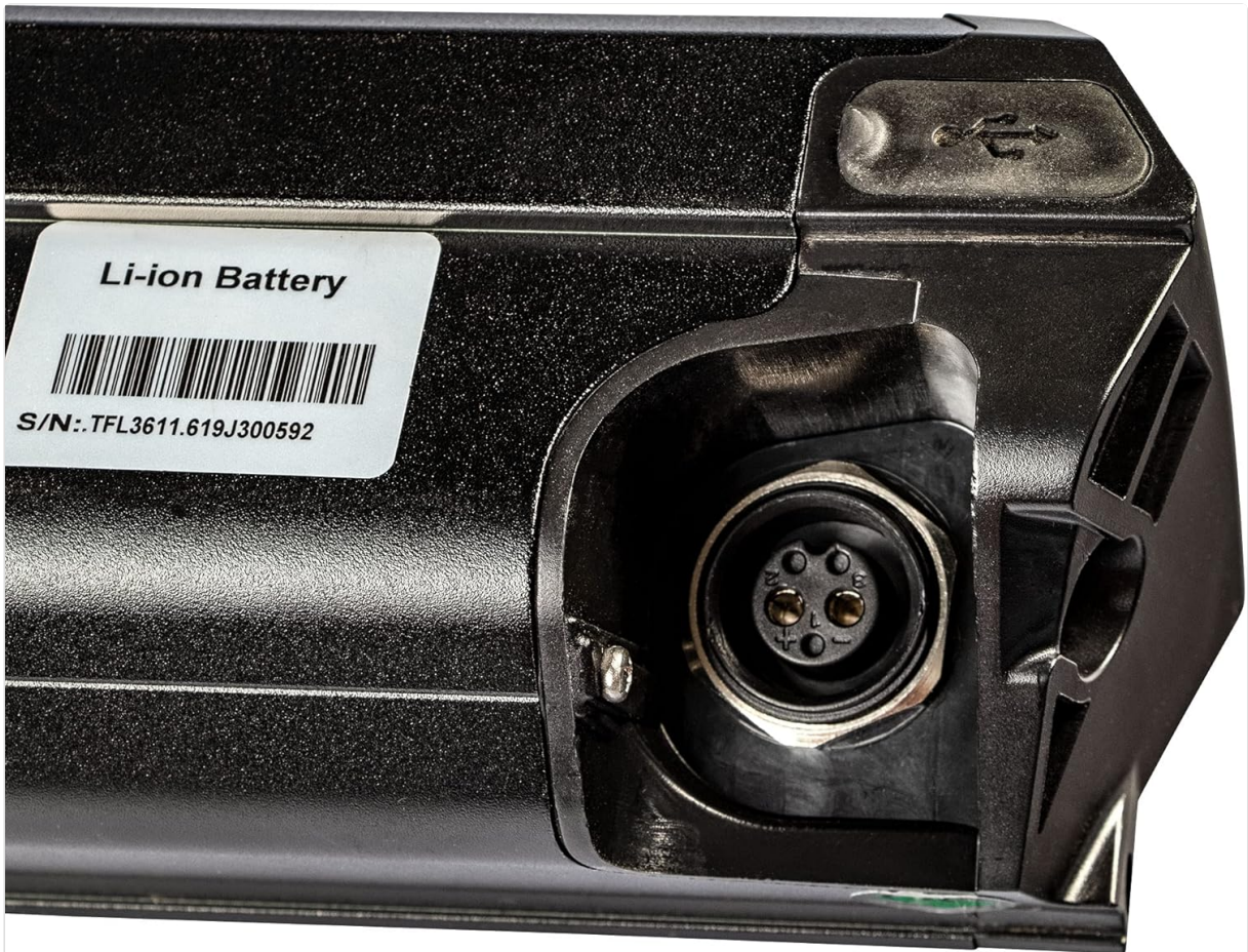
Figure 3.2: Close-up view of the battery's charging port and serial number label. The image highlights the circular charging connector and the white label displaying "Li-ion Battery" and the serial number S/N: TFL3611.619J300592.
