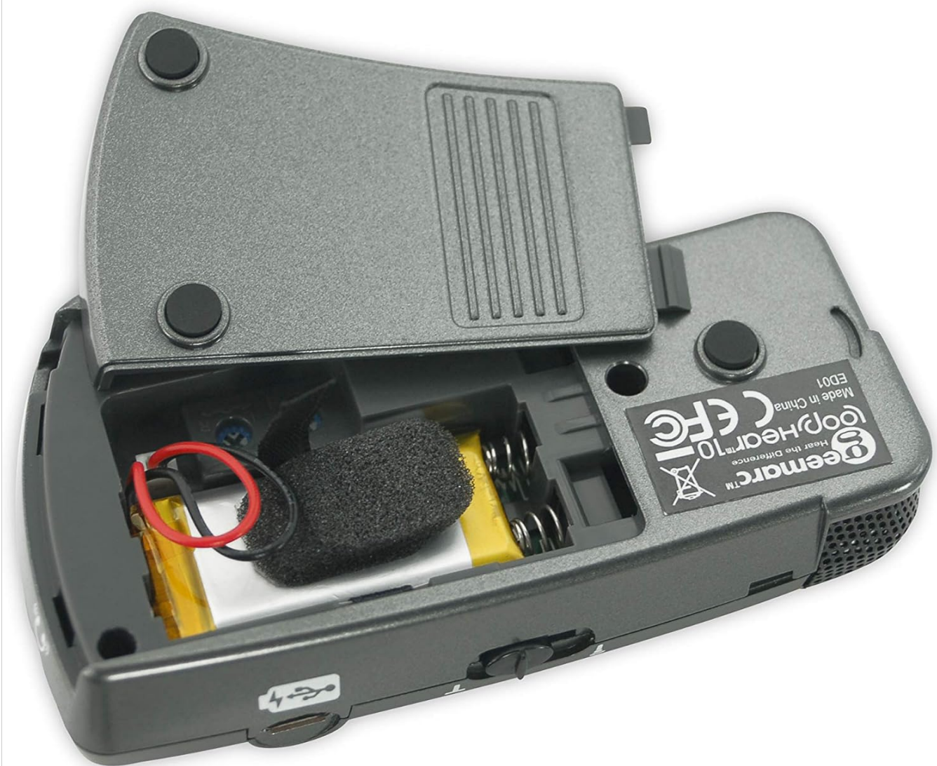
Figure 5: LH10 Battery Compartment. The underside of the LH10 unit with the battery cover removed, revealing the rechargeable Lithium Ion battery and its connection.
