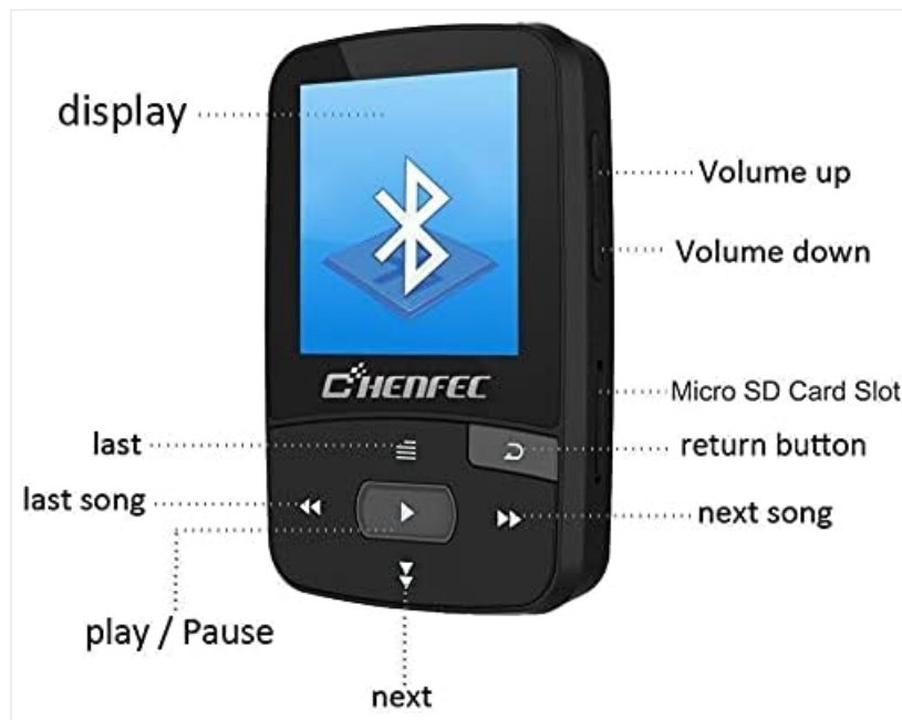
Image: A detailed diagram of the CHENFEC C50 MP3 Player, indicating the display, volume controls, Micro SD card slot, return button, navigation buttons (last, play/pause, next, next song, last song).
