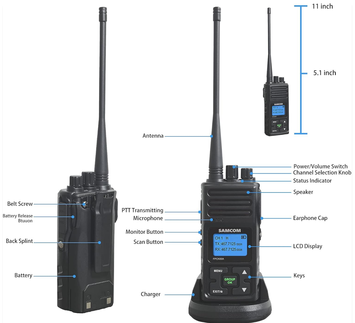
Image 3.1: Labeled Components of the FPCN30A Radio.
