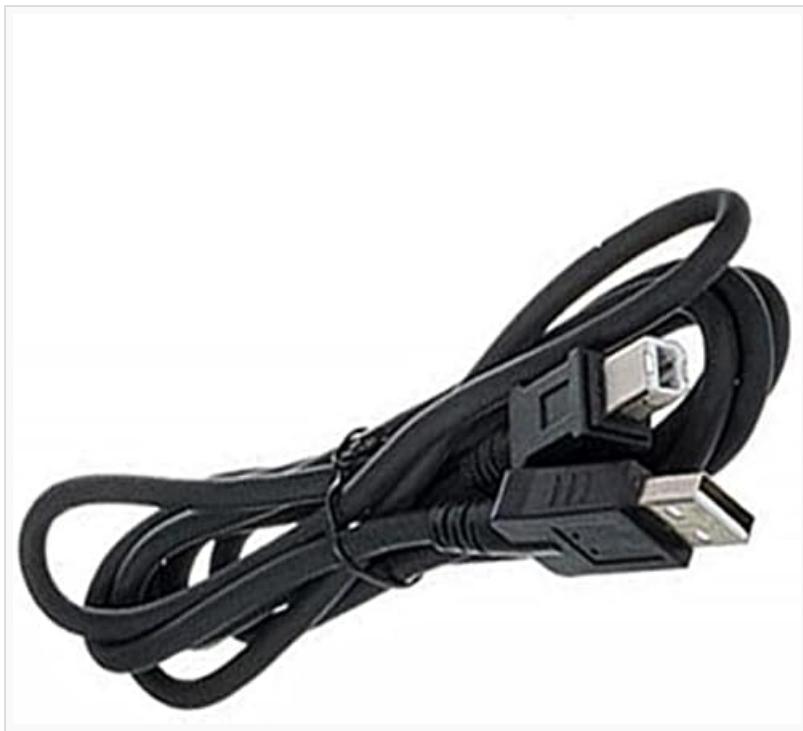
Image 4.3: The USB cable with a square connector for the microphone and a rectangular USB Type-A connector for the computer.
