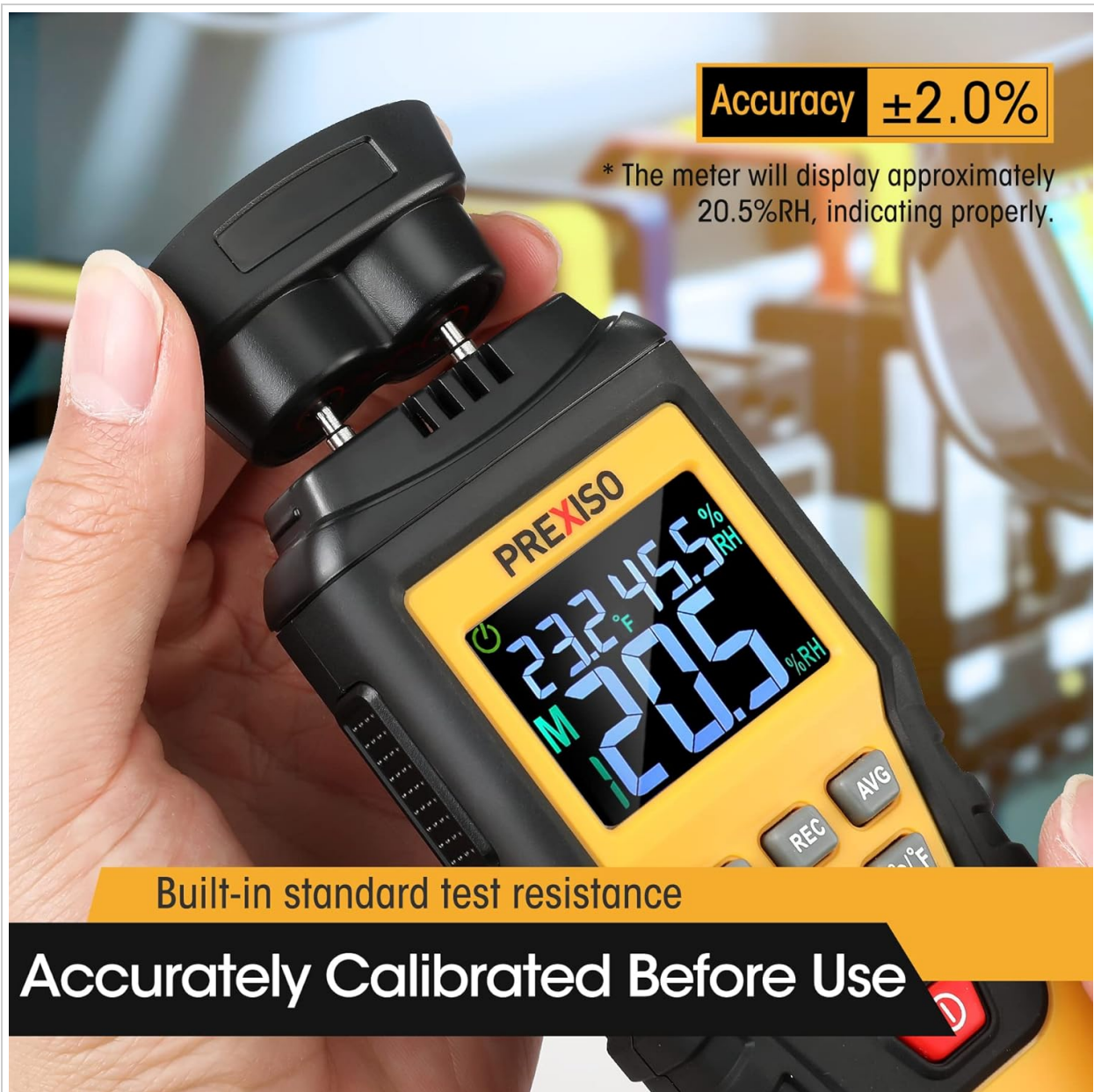
Image 3.1: The PREXISO PMX-57A Moisture Meter undergoing a calibration check by inserting the probes into the standard test resistance contacts on the probe cover. The display shows an approximate 20.5% RH reading, indicating proper function.
