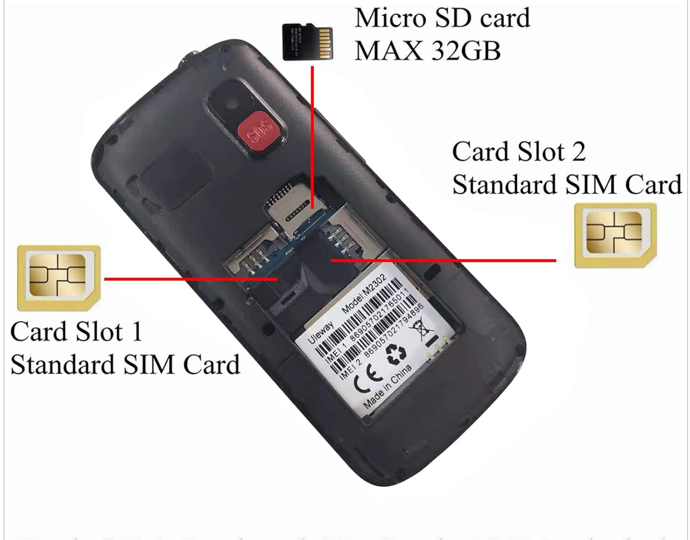
Image: Illustration of SIM and Micro SD card insertion points.
