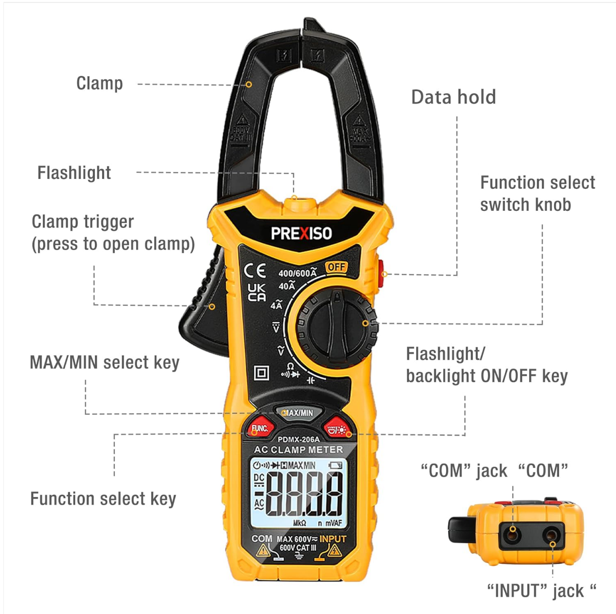
Image 3.1: Labeled diagram of the PREXISO PDMX-206A Digital Clamp Meter components.
