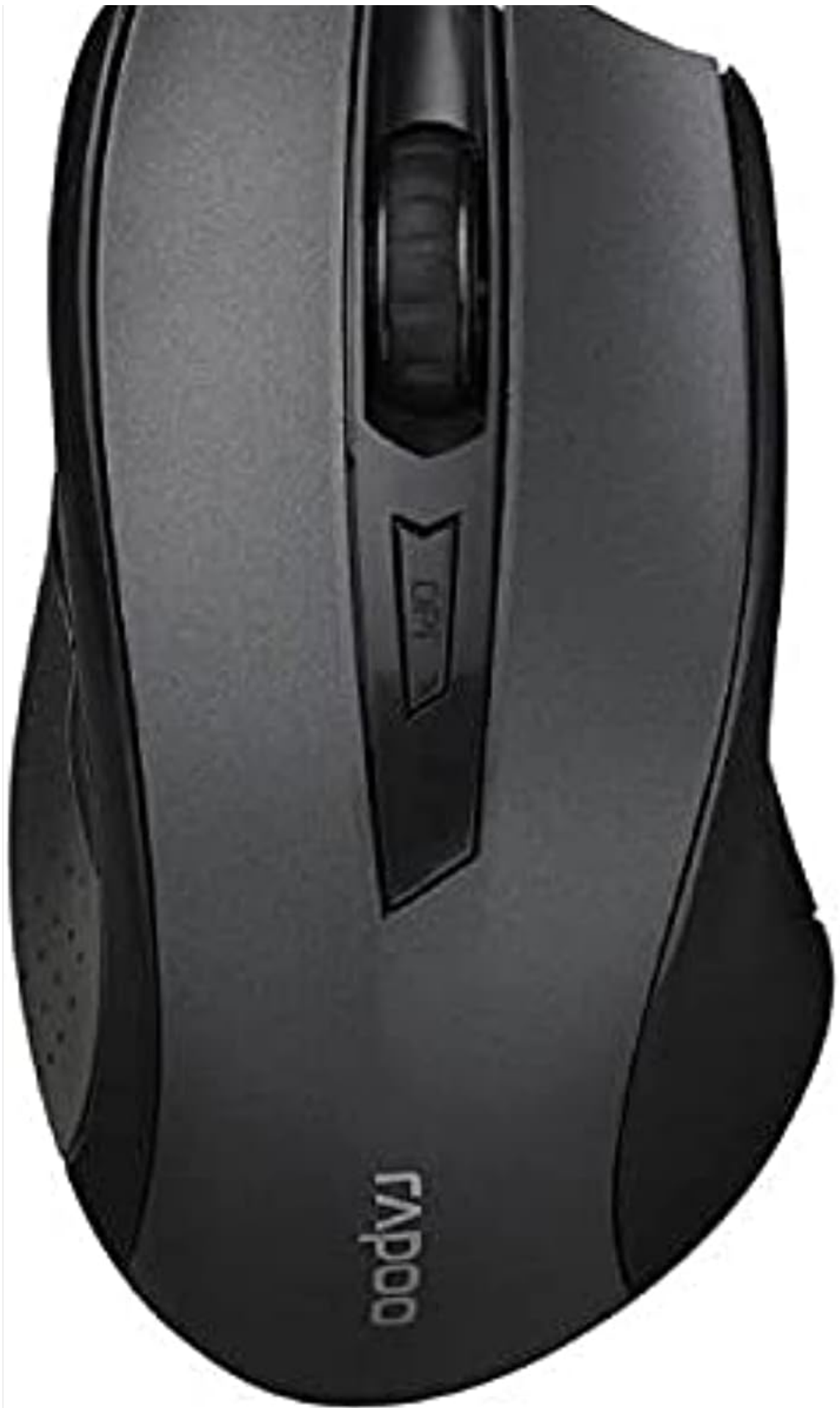
Figure 1: Top view of the Rapoo N300 mouse, showing the left and right click buttons, scroll wheel, and DPI switch button. The Rapoo logo is visible at the base.
