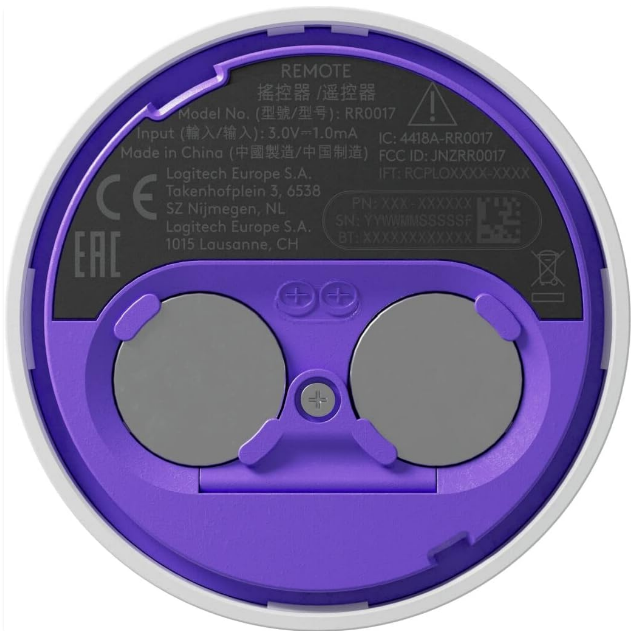
Figure 8: Underside of the wireless share button, indicating the battery compartment.
