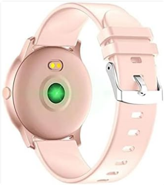
Image: The rear view of the REMAX RL-EP09 Smart Watch, clearly showing the two metallic charging contacts and the central optical sensor, which typically emits a green light for heart rate monitoring. This view is important for understanding charging and health tracking mechanisms.
