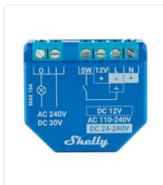
Image 4.3: Standard wiring diagram for Shelly Plus 1. L: Live, N: Neutral, O: Output, SW: Switch Input.
