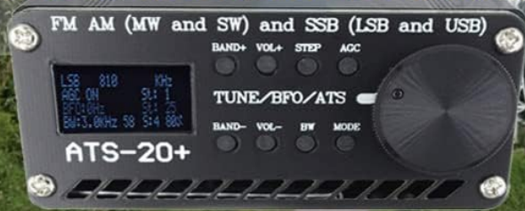
Figure 6: The display illustrating the wide range of supported frequency bands, including FM, AM, LW, SW, and SSB world band reception.
