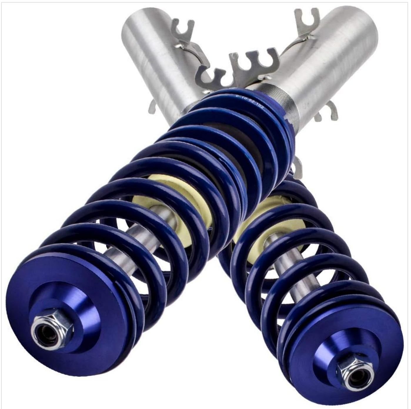
This image displays two maXpeedingrods coilover suspension units, featuring blue springs and silver-colored damper bodies, designed for vehicle suspension.
