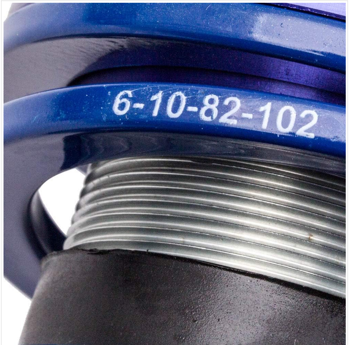
A detailed view of the coilover's blue adjustment ring, showing numerical markings (e.g., "6-10-82-102") used for precise ride height adjustments.
