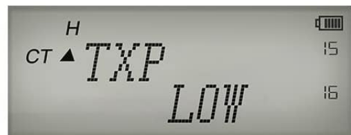
Image: The radio display indicating different transmit power levels: High (8W), Mid (4W), and Low (1W).
