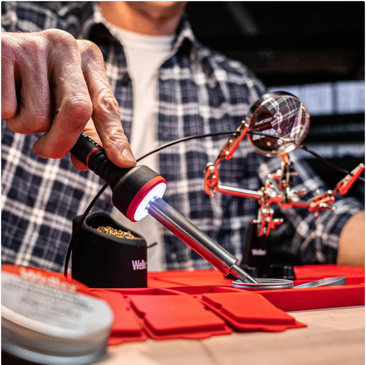
Image: Cleaning the soldering iron tip using a brass wool cleaner.
