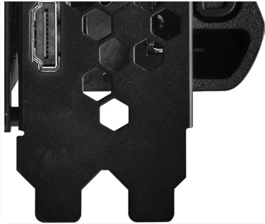
Figure 4.1: Graphics Card Output Ports (DisplayPort and HDMI).
