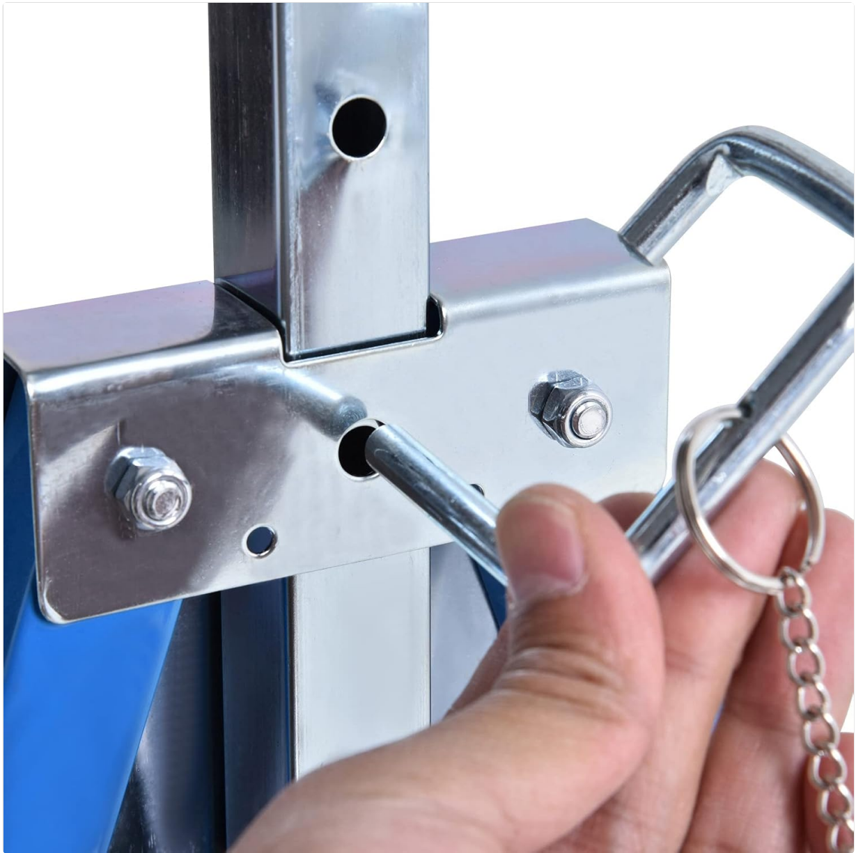
Image 4.2: Securing a Telescopic Leg with a Locking Pin
