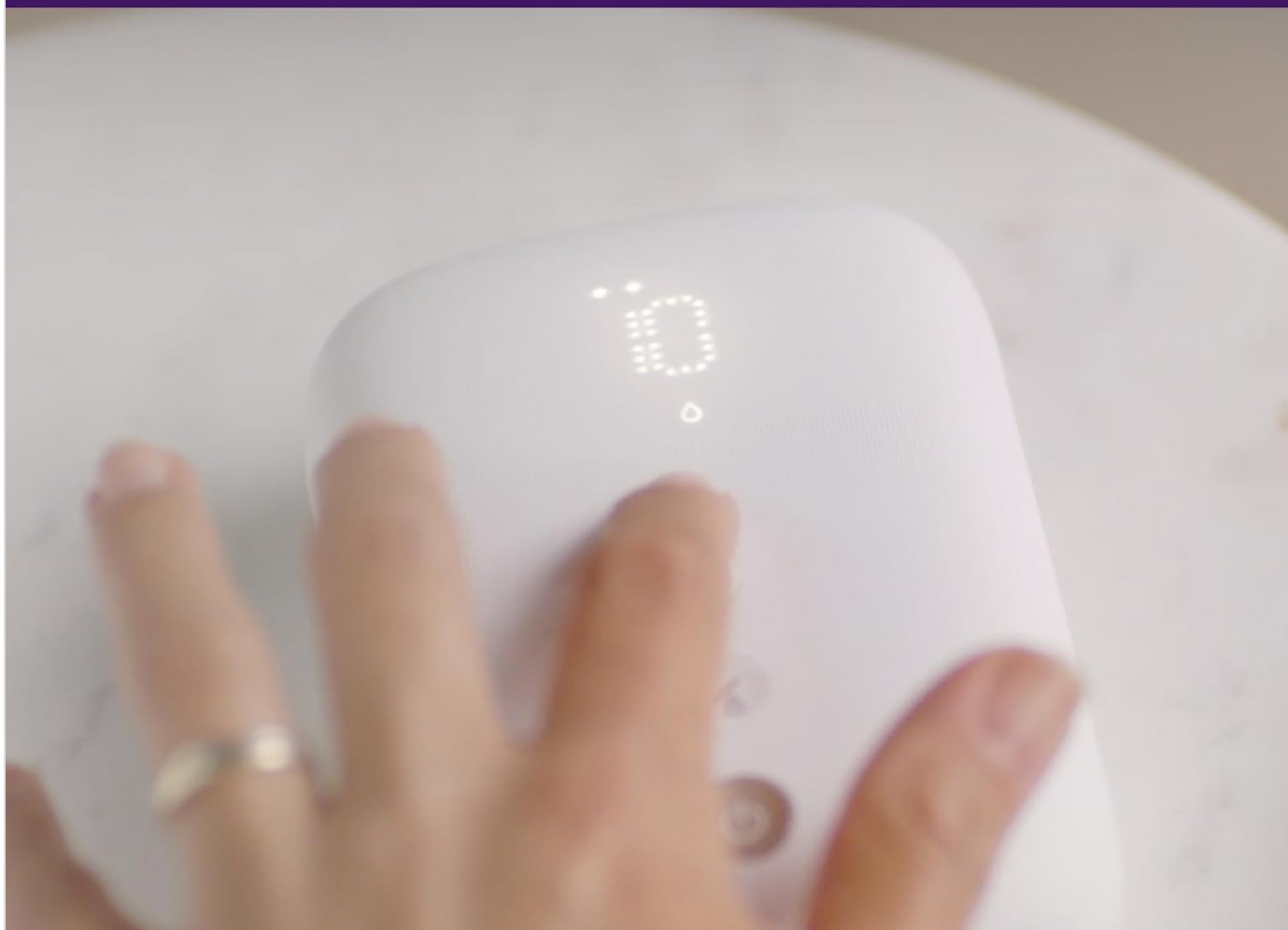
Image: Personalizing expression levels. The motor unit allows selection from 8 stimulation and 16 expression levels.
